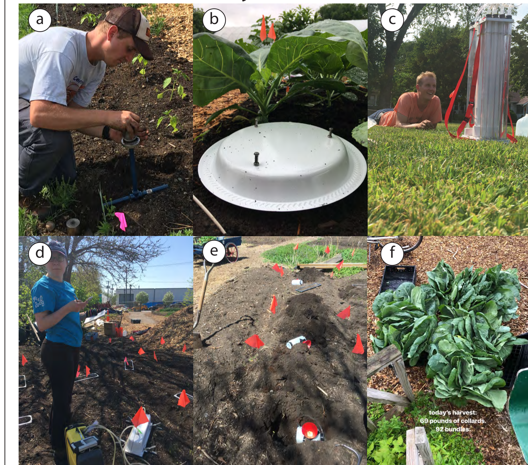
Figure 3. Making measurements of parameters relevant to ecosystem service evaluation. (a) Soil sampling (K. Buttel), (b) Pitfall traps to evaluate insect diversity, (c) Measuring saturated hydraulic conductivity (K. Buttel), (d) Gas flux measurements (J. Nicklay), (e) Lysimeter installation, (f) Crop yield and quality.
